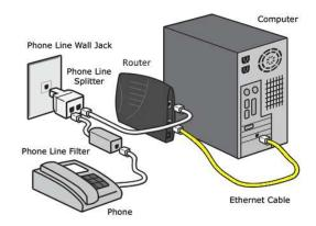
(Diagram above shows T-adapter and single filter. Dual filters, with T adapter built in, are also available for a minimal fee.)
